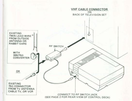
NOTE: If a VCR is already connected between the antenna and the VHF terminals on the back of your TV set, the RF Switch MUST be installed BETWEEN the VCR and
