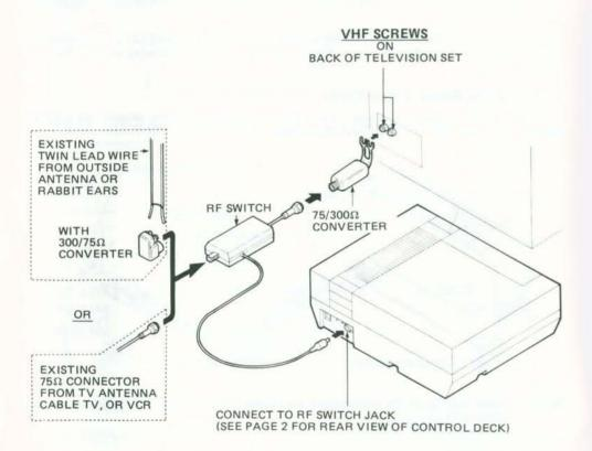
(ii) If your TV has a <u>VHF CABLE CONNECTOR</u> connect the RF switch and NES as shown below.
