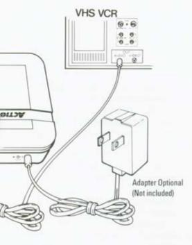
power adapter or a suitable power adapter coutput 9 VDC, 500ma, coax connector type (+) to center) to the base unit power jack. Batteries and the ACTIONMAX power adapter are sold separately and should be available where you purchased your ACTIONMAX game system.
